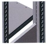
Insert the sides into the slots of the uprights starting at the bottom and following the panel profile.
